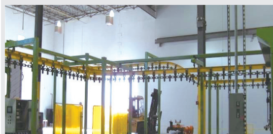
COIL 스프링 분체도장 Coil spring powder coating
