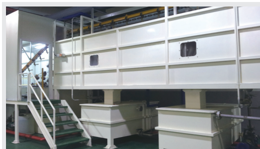
탕세, 탈지, 피막 Hot water cleaning, degreasing, coating
