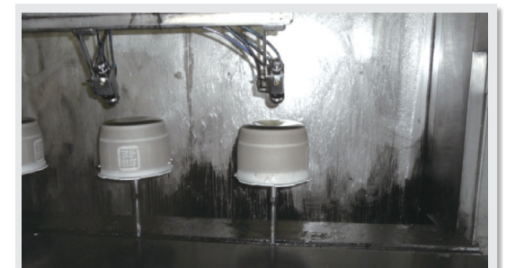
정밀회전 TEFLON COATING 장치 Precision rotation Teflon coating device
