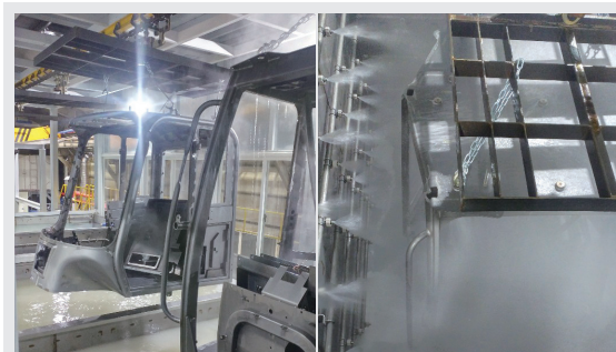
전착도장 Electrodeposition coating
