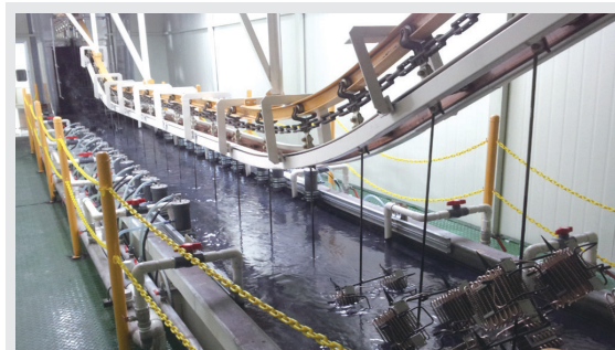
연속방식 전착 15TON EVA Continuous electrodeposit 15-ton EVA
